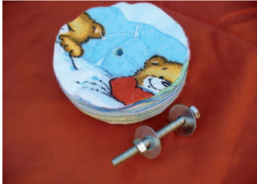
Clamping the polishing disc with FLEX polishing
